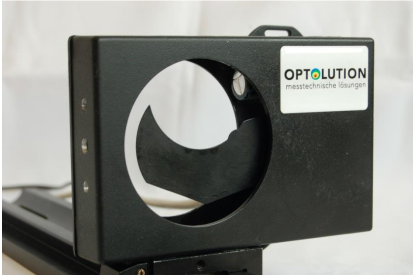
Front-view of the mechanical interlock laser shutter
