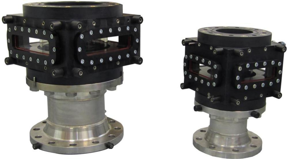
These window chambers from polyamide are **lighter** and produce **less reflections** than the stainless steel window chambers. They are manufactured from a single piece of material, which improves the mechanical strength. Our standard design is as following:
