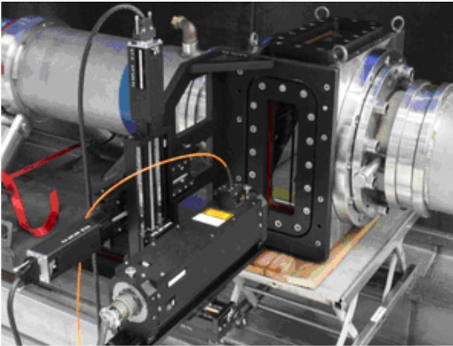
Window chamber produced for the PTB Berlin, Div. 7.5 Heat and Vacuum.
