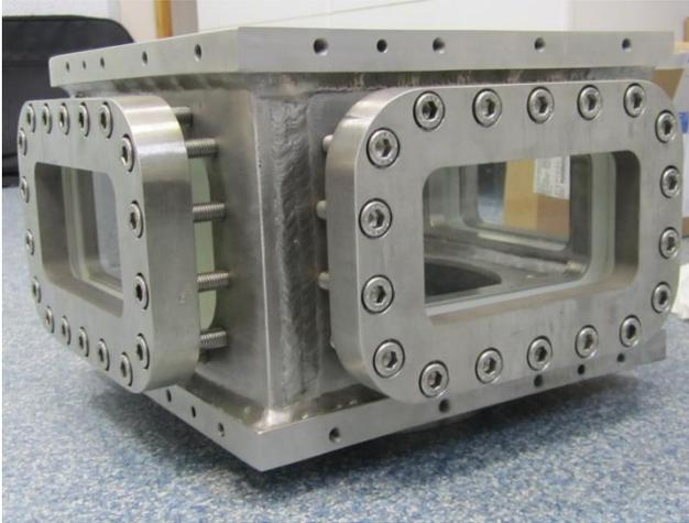
Solid layout of a window chamber used for a high pressure (10 bar) and high temperature (180°C) pipe flow. The application was the 2-component LDV measurement of the velocity distribution in the whole cross section. The typical window size is about 30 mm more than the tube diameter.
