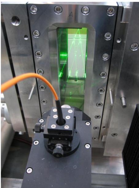
Setup for the investigation of a rectangular pipe flow. Due to the window on the opposite side LDV with forward scattering (e. g. Profile Sensor Technology) can be carried out in order to improve the spatial resolution of the boundary layer significantly.
