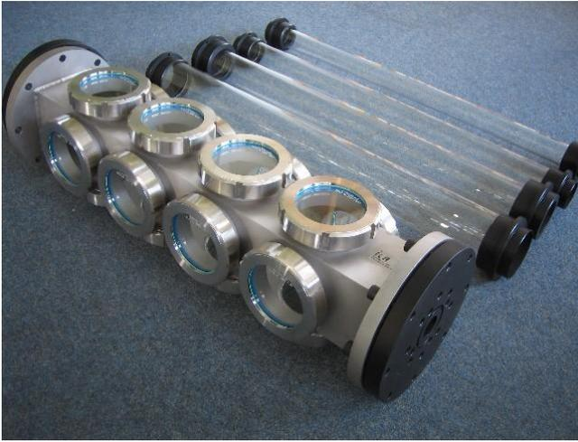
Window chamber with a rectangular cross section and a number of circular junctions. Model was used for studies regarding the flow distribution in a solar collector and to optimize the heat transfer.
