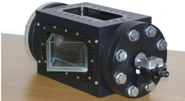
Similar design like above. The overlaying windows are used for **Stereo-PIV**. So the two cameras are located perpendicular in front of the glass pane and there is no lateral offset of the light by optical refraction.
