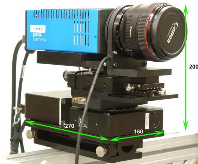
Complete motorised camera unit, with rotation, tilt, focus and aperture control
