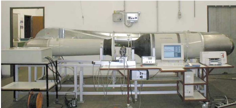
Test & Calibration wind tunnel equipped with LDV system
