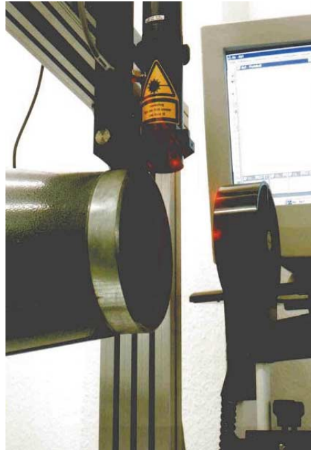
LDV probe mounted on a small open-jet wind tunnel, anemometer being calibrated
